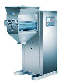
It is made of stainless steel. It's suitable for pharmaceutical, foodstuff, chemical, solid drink and other industries. It can make the stirred raw materials become granules with needed size or crush the blocked raw materials into small granules. The machine is mainly used for making granules with different specifications of pharmaceutical industry, chemical industry, foodstuff industry, etc.
