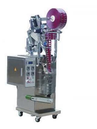
DXDF full automatic powder packaging machine is suitable for packaging powders of various densities. There are three sealing types for choosing: three sides sealing, four sides sealing and back sealing. With accurate measurement and easy cleaning, the equipment conforms to the national GMP standard. It has wide applications like pharmaceuticals, veterinary drugs, spices, mask powder, milk powder, pesticides, fertilizers packing.
