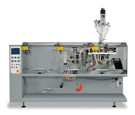
EM-130 Automatic bag packing machine is suitable for packing foodstuff. Pharmacy eutical pesticide, and daily using chemical etc. Different filling methods can be used for different products such as liquid, Powder, Granule and so on.
