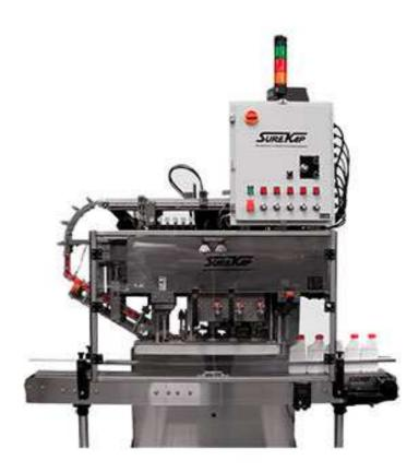
Based on a heavy duty stainless steel frame, our newest fully automatic capper utilizes the latest technology to automatically place and precisely torque a wide spectrum of cap types onto virtually any bottles type. The straight line, eight spindle capper features a new non-vibratory, high speed belt feeder with floor level loading and is designed for maximum efficiency and versatility.
