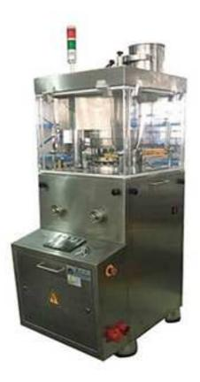
This machine is a continuous automatic tablet press for pressing granular raw materials into tablets. It is mainly used in pharmaceutical industry and also the chemical, food, electronic, plastic and metallurgical industries.
