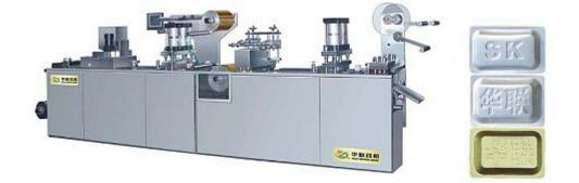
This machine mounts up forming and sealing of tropical aluminum on the basis of 250 blister packing machine. It takes on sealing moisture proof and light-avoiding entrance the value of product. It is widely used to pack all kind of products in pharmacy, food, medical health products, and medical apparatus etc. industrials.
