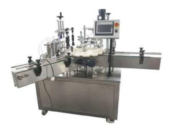
A semi-auto soft glue filling and capping machine is mainly used for glass bottle perfume filling and capping.
