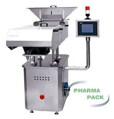
The counter PP-05 is a reliable, high performance machine, designed in conformance with current and proposed GMPs. Having a small footprint, they are effective in maintaining the integrity of a clean room environment. Few change parts are needed for different container sizes (only the nozzle). All product contact parts are made of type 316 stainless steel. And all contact parts can be easily disassembled for cleaning.
