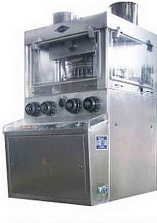
ZPW29/ZPW31 rotary tablet press is a double-press type continuous and automatic tablet press machine. It can press granular raw materials into round tablets, irregular tablets, double-layered and annular tablets. It could also press double colors and impress signs on both sides. The rotary tablet press is mainly used in pharmaceutical industry and also the chemical, food and electronic industries.
