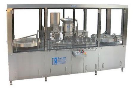
LAXMI Automatic Injectable Powder Filling & Stoppering (Full & Half bunging) Machine. The Basic Unit Consists Of One Or both side Turn Tables, S.S. Slat Conveyor Belt, Unique powder wheel. The Machine Is And Can Be Run Totally Through Touch Screen HMI, PLC Control And The Machine Is Based On Servo Motor Drive, The Machine Has an Output Speed of 120 Vials per Minute but Depending upon the Fill Volume and Container Dia. /size Or the Quality of Powder
