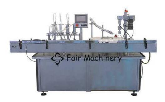
It uses a microcomputer to set the number of steps peristaltic pump to perform metering filling, and is used for the production of a new generation of daily chemical and pharmaceutical pastes. Products required by GMP. It can also be used for small-dose liquid filling and capping production in other industries.
