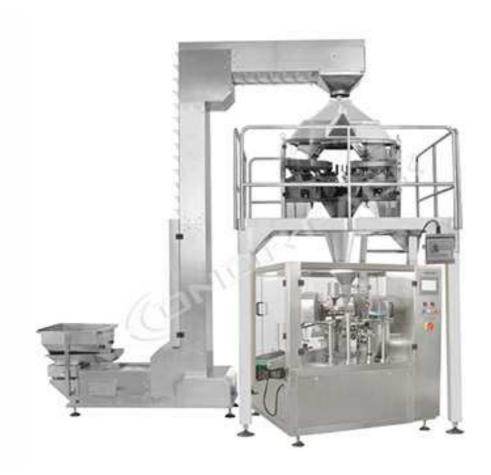
Equipped with Z-shape bucket elevator and combination scale, it is widely applied to candies, microwave popcorn, cookies, nuts, rice, coffee beans, crops, peanuts, etc.
