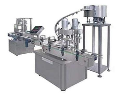
This machine has the function of automatic bottle charging, positioning, filling, cap charging and screw-capping and can be used in paramedical, food, cosmetic, chemical and other industries.
