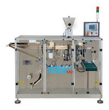
YODM/180 Sachet Packaging Machinery is full automatic machinery with PLC control which designed for producing 3 or 4 side sealed packs. Filing System for the machine produces as Volumetric, Auger (Screw) and/or Liquid filling system according to the products to be packed Filling volume of the machine is between 10-200 ml The main usage area for this machine is to pack products like spices, sauces, soup mix, tea, coffee, cream, ketchup, mayonnaise, yeast powder, shampoo, etc.
