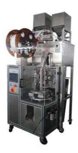
Be able to measure; make bag, fill, seal, cut, print date automatically.
