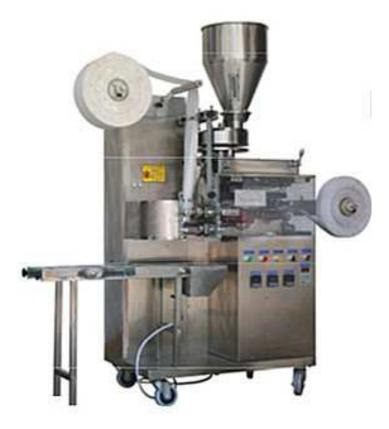
BT-11 is a heat-sealing, multifunction; automatic, intelligent tea-bag packing machine. The machine can automatically finish bag making, filling, seal of the tea bags, and attaching the string and the tag.
