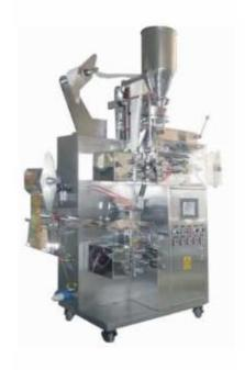
STB-10A automatic teabag packing machine is specially designed for tea, herbs, coffee as well as other drinkable products in the filter bag with an outer bag. It's an auto-weighing filling and bag forming sealing. Widely applied in the market of chemical powder, food powder, additives, this machine unit has been accepted by customers for long time.
