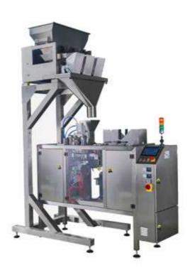
Function: preformed bag picking-up, opening, filling and sealing, or premade pouch pick open fill and seal
