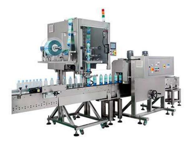
Auto Body Label Sleeve Applicator, LF-100 can be installed perforation device to punch varied perforating pattern such as vertical, horizontal, L-type or V-type lines. It is designed with SUS frame to match production requirement of Foods & Pharmaceutical industries. Also, machine could be installed remote control feature to monitor production.
