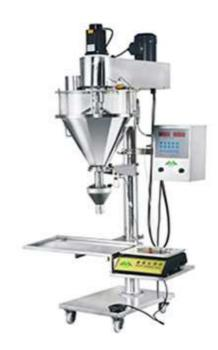
This Milk powder screw filling machine adopts screw filling and electronic weighing feedback measurement method, and combined with PLC control.
