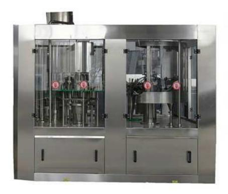
This Automatic Beer Filling Capping 2 In 1 Machine is mainly used for glass bottle crown caps of beer filling and sealing. It is 2 in 1 machine, composed of beer filling and crown capping. The machine adopts international advanced technology, it's design scientific and reasonable, appearance is beautiful, operation and maintenance is convenient, and it's high degree of automation, so it is the good machine for middle and small beer manufacturer.
