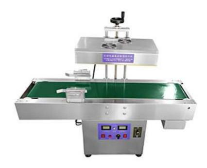
This automatic electromagnetic-induction aluminum foil sealing machine is suitbale for Bottles, Containers, Cans and Jars. Its non-contact heating feature is suitable for sealing the mouth of plastic containers. The material of the plastic container can be: polyethylene (PE), polypropylene (PP), polystyrene (PS), polyester (PET), polyvinyl chloride (PVC), ABS, etc. However, metal bottles and metal caps cannot be sealed.
