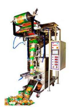
Automatic Pouch packing machine Double head weigher is developed for precise and high-speed quantitative weighing packaging system. Linear Weigher is suitable for weighing materiel of small grain with good uniformity, such as oatmeal, sugar, salt, seeds, rice, sesame, milk powder coffee, etc. Also available in single, two, three& four head.
