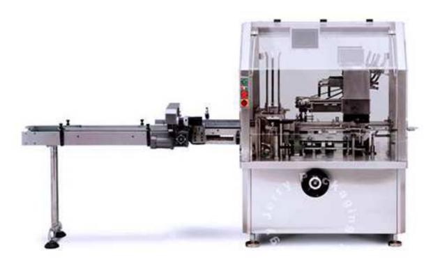
This machine completes product insertion, leaflet insertion and production batch & expiry date coding in one run. Also equipped are malfunction warnings for fail safe packaging processes. It is labor saving, suitable for pharmaceutical, ointment or cream tubes, cosmetics, hardwares, stationary, etc.
