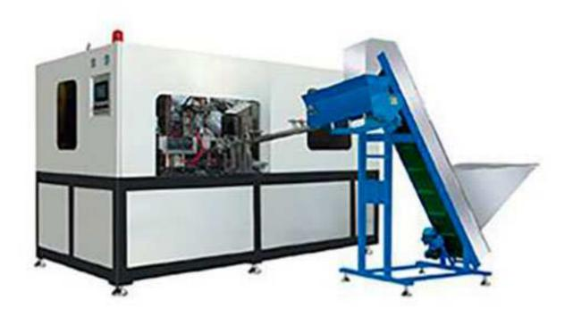
SKS-2000 Plastic water bottle blow molding machine is controlled by PLC. The whole process from preform feeding to bottle discharging is completed automatically with advantages of labor saving and no pollution. HY-2000 consists of three main parts: preform loading system, Heater channel & blow station.
