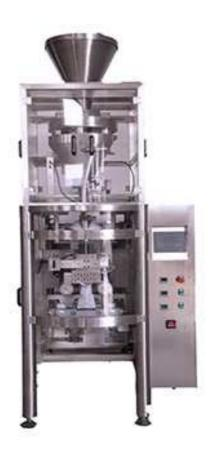
VFFS vertical packing machine suitable for salt, sugar, sesame, rice, seed etc even granule material packing. Including bag forming filling and sealing.
