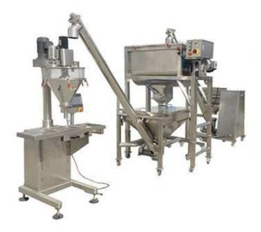
The dry powder mixing machine is a new type, high efficiency mixing equipment, are widely used in food and chemical industry. Horizontal tank body, need small space but more capacity.
