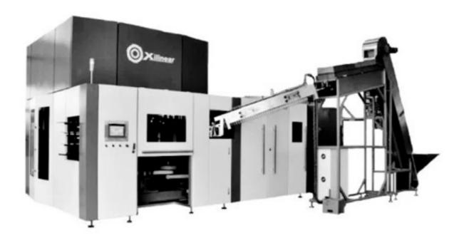
6 Cavity Rotary Blowing Machine a plastic processing machine. Its working principle is that the tubular plastic parison obtained by extrusion or injection molding of thermoplastic resin is placed in a split mold while it is hot. The compressed air is injected into the parison immediately after the mold is closed to inflate and tighten the plastic parison. Stick it on the inner wall of the mold and release it after cooling to obtain various hollow products.
