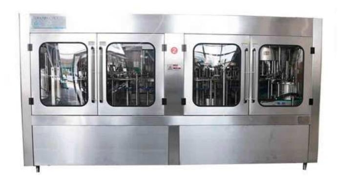
Our newly designed DCGF serious monoblack carbonated drink filling machine is designed for bottle filling, it can suit for PET bottle and glass bottle size between 150ml to 2000ml, can customized to maximum of 3000ml. Genus design of capping design makes different screw cap change into one simple easy torch. On machine surface is only leaving 3 points of bearing support point which makes drainage so easy and without any dirt stain.
