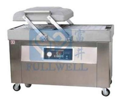
CE series Double chambers vacuum (aeration) packaging machine, As long as you press the vacuum case's lid, the machine will automatically complete the orderly assumed processes of vacuum extraction or aerate the orderly assumed processes of vacuum extraction or aerate the inner gas, sealing, printing, cooling and aeration. The packed products can be prevented from oxidation, going mould, insects or getting damp, thus can be kept fresh in a prolonged storage period.
