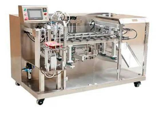
The horizontal premade pouch machine can fill and seal custom premade pouches at one time, such as stand up pouches, flat bottom pouches, gusseted pouches, and quad seal pouch. Based on the type of products, and the target packaging weight, the single lane premade pouch packing machine can complete 30-60 bags per minute.
