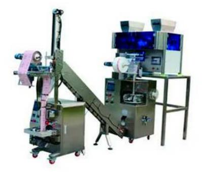
This machine is used to package tea as flat bag or pyramid bag. It packages different tea in one bag.
