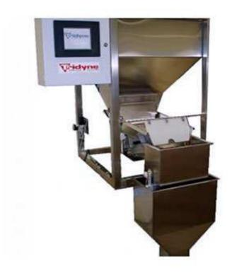
The Tridyne F-100 Series of Net Weigh Fillers are available in 4 different configurations. It can be used as a table top model or can be integrated with other industrial bulk filling equipment such as baggers, conveyors, sealers, and more. Products need to be free flowing.
