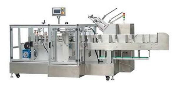
The cartoner Machine automatically picks the carton and forms the carton, worker manually puts the products on the moving conveyor, and when it's moving to the formed carton, the machine pushes it into the carton, sealing the carton with glue. If you want to save the labor cost, you can add a robot to place the goods on a conveyor instead of one person.
