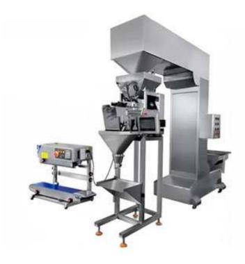
Linear weigher is suitable for weighing slice, roll or regular shape products such as sugar, salt, seed, rice, sesame, glutamate, milk powder, coffee powder and seasoning powder, etc.
