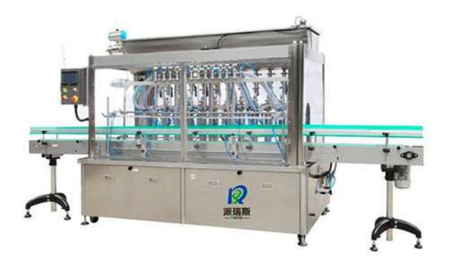
This type of machine is suitable for semi liquid and cream without gas. It automatically count inlet bottles, quantifiably fill each bottle, and deliver outlet bottle. It is especially good for filling SL, EC, SC, Edible oil, lubrication. This filler is an idea choice for foodstuff, pharmacy cosmetic chemical, and pesticide factories.
