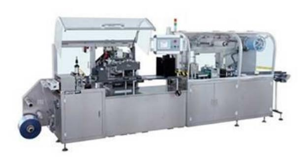
The machine feeder can be connected with labeling machine and output can be used with cartoning machine, thus forming a complete automatic packaging production line. Equipped with PLC and HMI touchscreen control system. Uses servo motor-driven and the main motor adopts frequency control. With special automatic servo drive feeder for ampoule, vial and pre-filled syringe. This machine is equipped with blister forming detection, feeding detect rejection, safety cover, and chiller cooling system.
