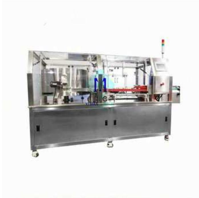
The Bottle Unscrambler Machine is used to automatically orient and feed containers into the production line. It can unscramble plastic, metal, and other non-fragile containers.
