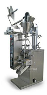
The machine is designed and manufactured specially for powdery and super fine powdery products Driven by servomotor, the auger is rotating to fill products; furthermore, the filling range can be adjusted automatically through computer. The processes of bag making, measuring, filling, sealing, cutting, counting and hot pressing codes can be done automatically.
