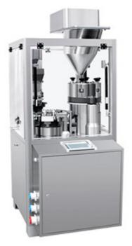
NJP-800 Fully Automatic Capsule Filling Machine is filled by powder, grain, and tablet. It adopts multi-bore dosing, intermittent motion and timing frequency conversion. It is suitable for automatically completing capsule feeding, separating, filling, (waste capsule rejecting), closing, finished product ejecting for powder or tiny pill medicine in capsule. It is designed sophisticatedly by our factory according to the practice on domestic; it is fully accord with the GMP standard.
