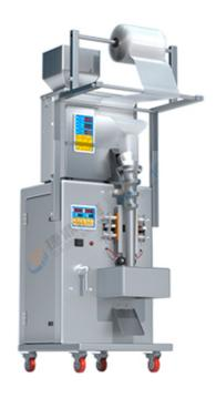
The 200g electric small packing machine produced by JD is suitable for the quantification, weighing, filling and sealing of rice, millet, cereals, vegetable seeds, cat food and dog food, fertilizer feed, nuts and seeds, corn seeds, coffee beans, coffee powder, flour, pepper powder, seasoning powder and other particles, powders and materials
