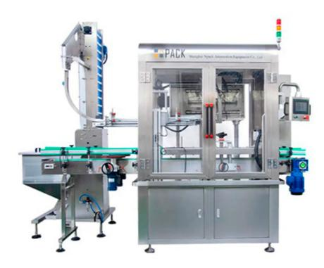
The Automatic Tracking Capping Machine represents a technological breakthrough for the packaging industry, perfectly complementing the automatic tracking filling machine to create a comprehensive packaging line solution. Featuring an advanced motion controller, all of its operations are powered by servo motors, making it a near-fully intelligent piece of equipment. This innovation ensures unparalleled precision and efficiency, marking a significant step forward in automated packaging processes
