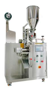
This type of small vertical packaging machine is an upgraded model of CB-280, packing speed up to 100 bags per minute.
