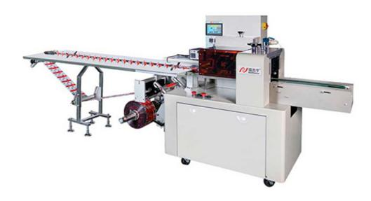
The automatic dry fruits packaging machine ZP-3000S adopts industry-leading electronic cam algorithm, and the bag lengths range from 90mm – infinite. Once the bag length is determined, it can be cut in one step, saving time and film.
