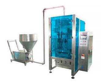
Equipped with input pump, the machine could automatically pack the products in high temperature that will improve the productivity, decrease the cost, and avoid making the twice packing. Full automatic liquid / paste products quantitative bag packaging equipment is widely used in packing filling of sweetened bean paste, filling of lotus meat, fruit jam, Chinese watermelon jam, cheese jam, sauce, salad, lotion, liquid, semi liquid.
