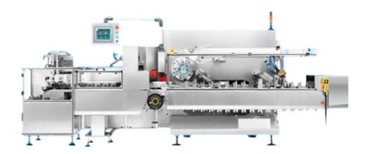
Can complete the following functions automatically: Feeding, Leaflet folding, Carton opening, Blister inserting, Leaflet inserting, Batch number on cartons, Cartons sealing, etc.
