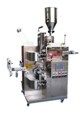
It is suitable for automatic filling and metering of soft bags for tea, Chinese herbs, coffee and so on. It can realize packing of inner and outer bags, hanging thread and hanging tag.
