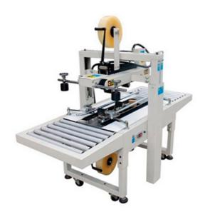
FXJ-6050 is operator fed and designed for heavy duty applications. These machines are reliable, cost-effective and durable providing savings to your production process. More importantly, these machines provide a professional looking seal. The FXJ-6050 Semi-Automatic Uniform Carton Sealer with Easy Manual Carton Size Adjustment has a 4-belt design (2 top and 2 bottom). The machine comes complete with infeed/exit conveyors, casters, power cord, and plug.
