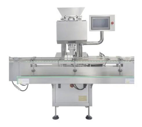
This machine is a intelligent automatic counting and filling machine, which is widely applied for capsule counting for big scale production in hospital, pharmaceutical factory etc.
