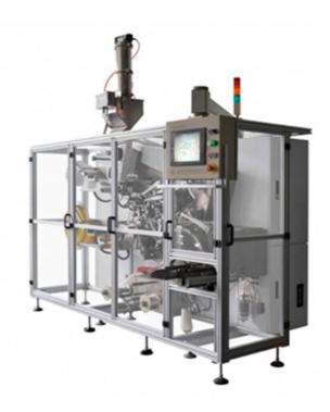
The machine SG-10 is a kind of automatic tea bag machine for the packing of tea and similar Chinese herbs / Flower tea. It makes double chamber tea bags which are cold-sealed. The machine links up hard label and thread with staple, and the tea bags are pushed out and packed into box manually after counting. The packing materials are non-heat-sealed filter paper, label, thread and staple.
